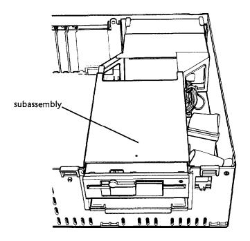
To remove the subassembly, first lift it up from the front only. Place your thumbs under the diskette drive and grasp the top edge of the computer with the rest of your fingers, as shown in the next illustration. (If you have a diskette drive installed in the lower horizontal drive bay, place your thumbs underneath that drive instead.)
